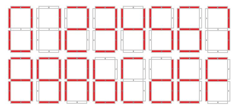
The image above represents the entire hexadecimal character set [0-9, AbCdEF] for this particular seven segment display. Note that the digits 'b' and 'd' appear as lower-case letters to avoid the ambiguity with the digit 8 and 0 respectively. A special character where no segments are on can be used as a space.
