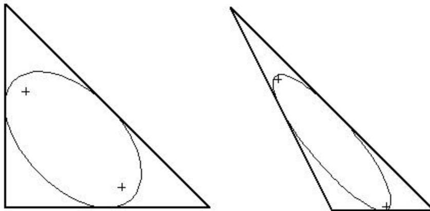
Joe knows how to draw an ellipse by putting two stakes in the ground (at the foci of the ellipse), tying a rope between them and dragging a marker stick inside the rope. What Joe would like is for the customer to determine where the corners of the triangle will be and then measure the location of the triangle vertices and compute where to put the stakes and how long to make the rope.
